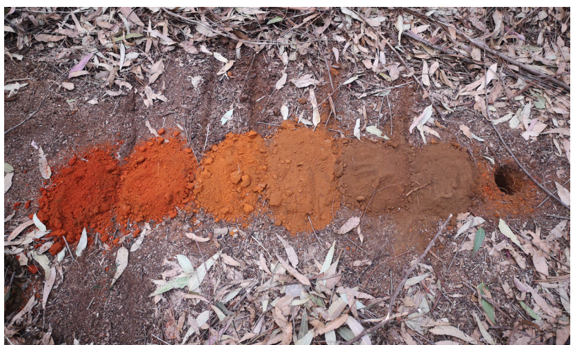
Figure 1: Soils samples are taken just outside the four corners of the plot, at three depths, and analysed at the ICFR analytical laboratory facility.
