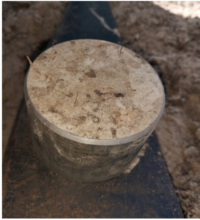
Figure 3: Soil bulk density samples are taken to determine important soil physical properties at each site.
