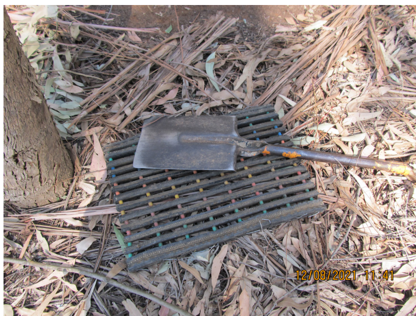
Figure 2: Litter samples are taken using a 30 cm x 30 cm grid where soil samples are also taken and analysed to quantify levels of N, P, K, and other macro and micro nutrients.
